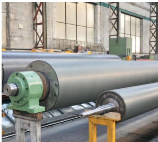
Ceramic-coated wire drive roll and wire guide roll from the wet end of a paperboard machine
