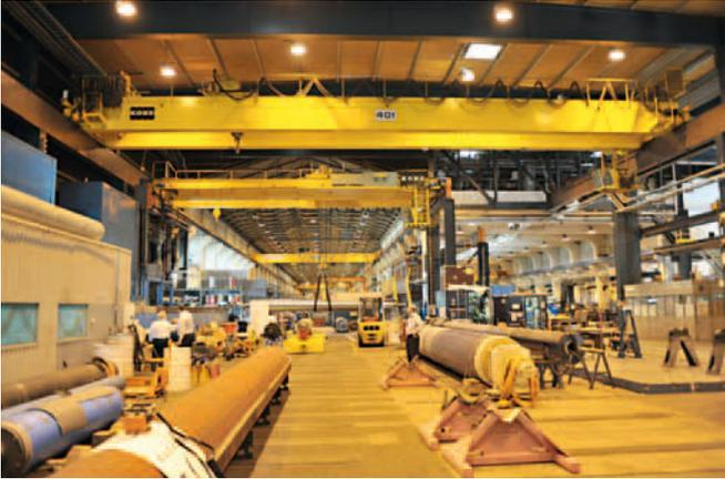
The production consists of four hall naves. Each nave is optimized in production technology for certain roll types and roll sizes
