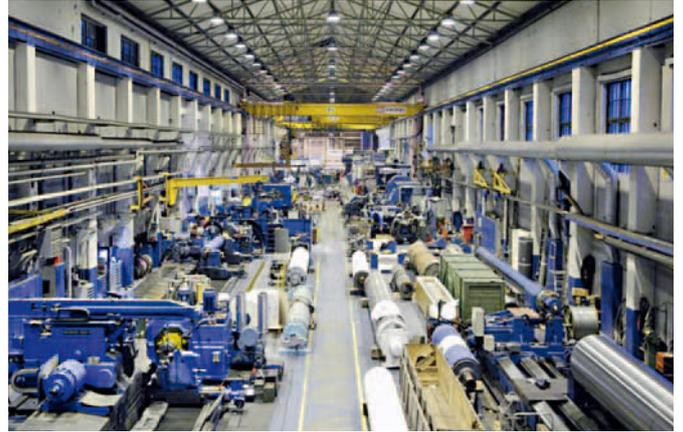
Hall nave for processing large rolls, e.g. lathing, beveling, drilling holes, honing and balancing. Here, piece weights of up to 80 tons can be processed.
