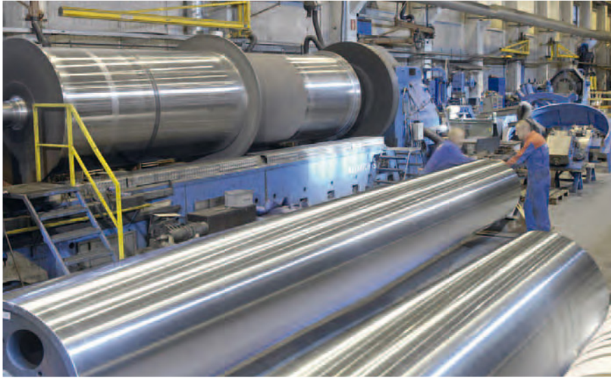
Large rolls turning shop in Karhula factory for max. components sizes 2.10 m diameter x 18 m length (80t)
