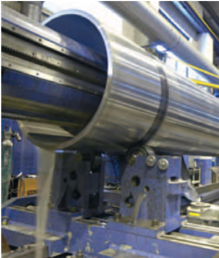
Drilling out a pipe for the production of a new deflection compensating roll
