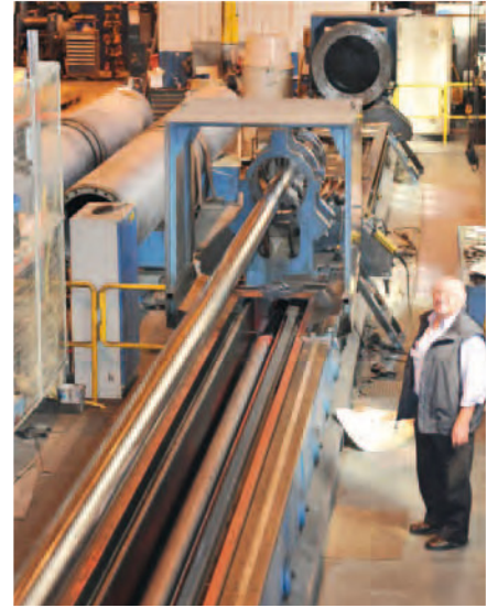
Wolfgang Richter at the honing machine in Karhula. Diameter 1.70 m x 10.50 m length (60t)
