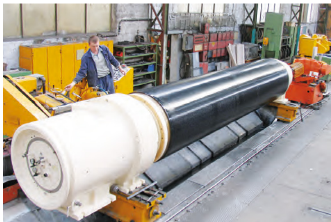
Grinding with a generally overhauled suction roll in Plant II rolls
