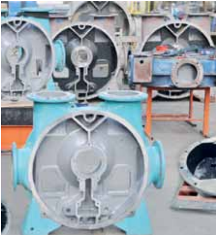
Side brackets coated with the composites that are adjusted to the relevant use conditions
