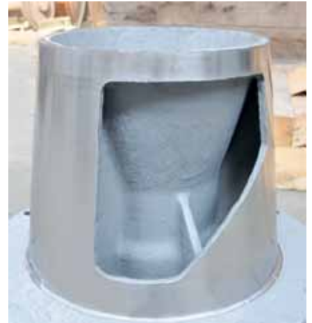
Cleaned Nash cone which was additionally coated with composites protecting against new deposits
