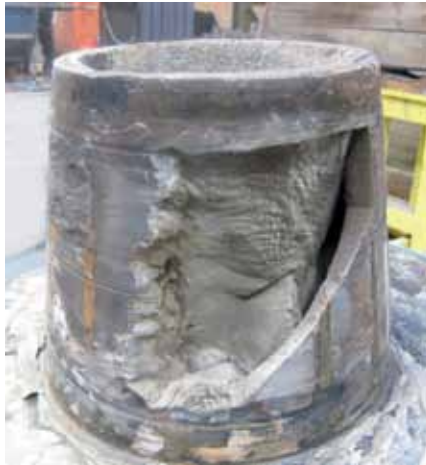
Clogged Nash cone, the on-site analysis showed an 85% loss of performance
