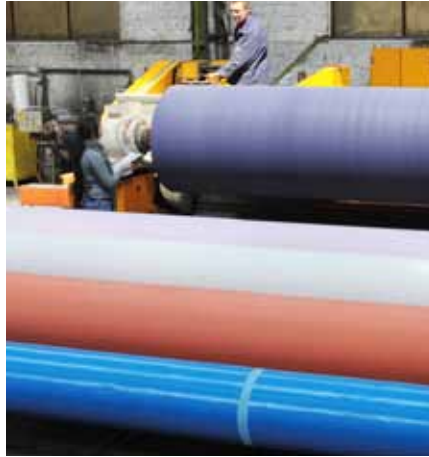
RiWaMat Composite Ceramic Cover op de slijpbank
